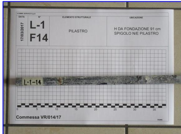
Foto 31: Barra prelevata in L-1 - 14
