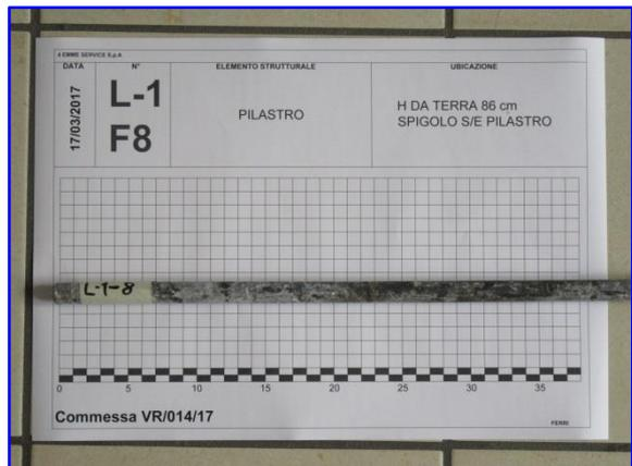
Foto 29: Barra prelevata in L-1 - 8
