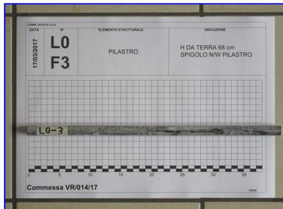
Foto 35: Barra prelevata in L0 - 3
