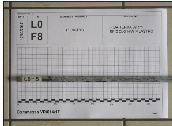
Foto 37: Barra prelevata in L0 - 8
