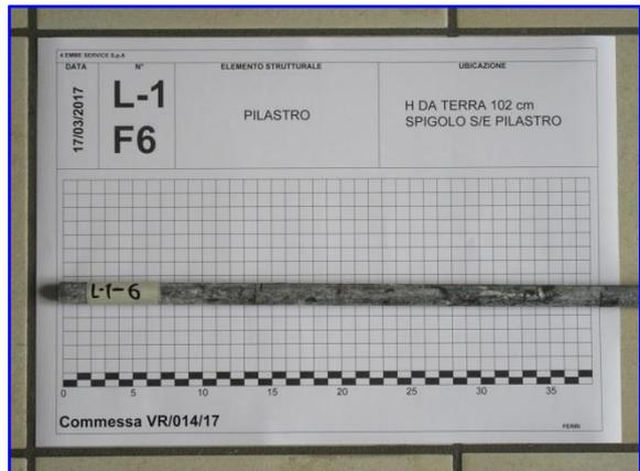
Foto 27: Barra prelevata in L-1 - 6
